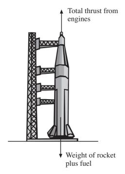
The rocket is powered by 3 engines **each** of which produces a thrust of 2 000 N. The mass of the rocket and its fuel is 500 kg, so that its weight is 5 000 N.
