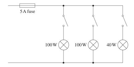
Use the information in the table to find the current flowing through the fuse when all these lamps are switched on. [2]
