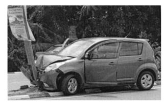
The front of the car was designed to collapse to protect the driver and passengers.
