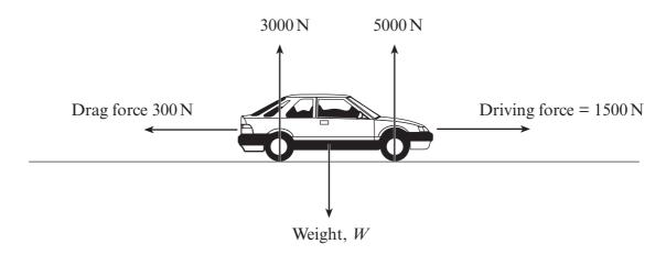
(a) The vertical forces are balanced. Write down the value of W. [1]
