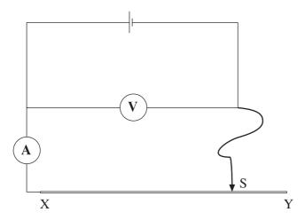
(a) With S in the position shown, the voltmeter reads 6 V and the ammeter 1.2 A. Use the equation
