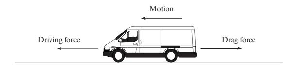
The driving force is  $1000\,N$  between 0 and 20 s. The mass of the van is  $2400\,kg$ .
