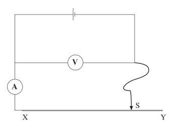
(a) With S in the position shown, the voltmeter reads 6 V and the ammeter 1.2 A. Use the equation
