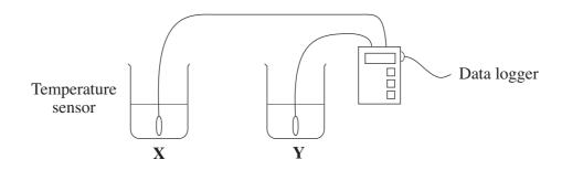
The students filled the cans with the same amount of hot water. A data logger was used to record the temperatures.
