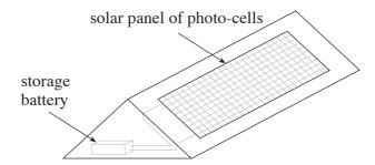
On a typical summer day in the UK, the solar radiation received at the panel is 6000 W (in the absence of cloud). The efficiency of the panel in converting solar power to electrical power is 20%.
