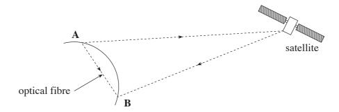
(a) Information is passed from **A** to **B** using a satellite in geosynchronous orbit  $3.6 \times 10^4$  km above the Earth's surface. Microwaves carry the information at a speed of  $3 \times 10^8$  m/s from **A** to **B** via the satellite.
