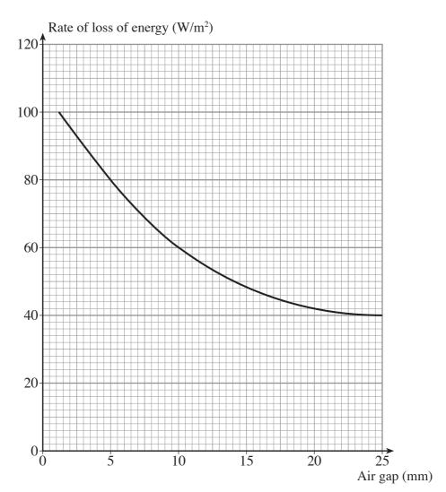
(i) Describe how the rate of loss of energy is related to the air gap. [2]
