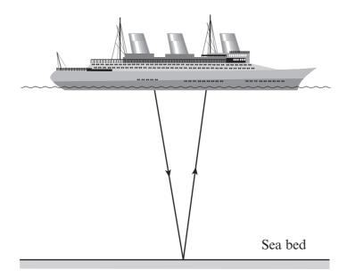
A wave is sent out from the boat to the sea bed and is received back 3 seconds later.
