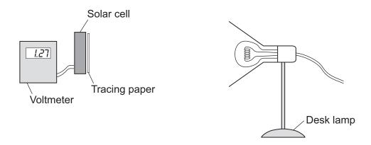
The student put the desk lamp a fixed distance from the solar cell. To represent the effect of a dirty surface, the student covered the surface of the solar cell with pieces of tracing paper. Each time the student added a piece of paper, she measured the output voltage of the solar cell.
